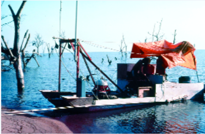
Figure 8. Catamaran used for gravity acquisition on Lake Rukwa, Tanzania, 1983. The underwater gravity meter is the round object in the center of the boat.
